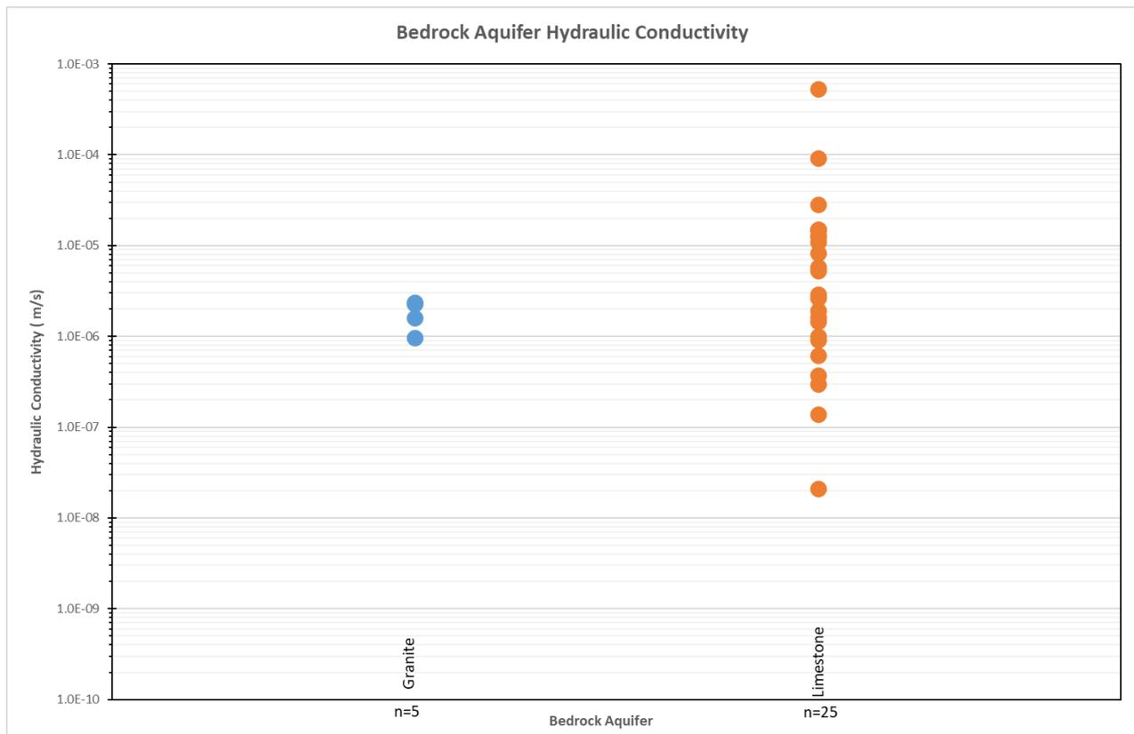
**Plate 10.1 Distribution of Calculated Hydraulic Conductivity**
