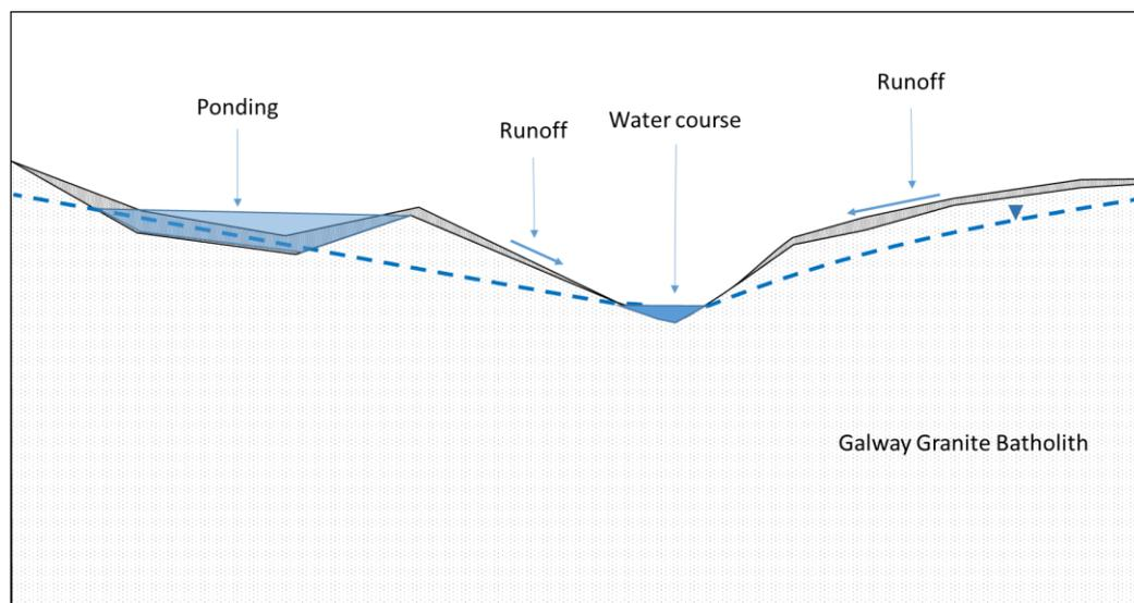
**Plate 10.2 Hydrogeological Conceptualisation of Runoff and Surface Water Ponding on the Galway Granite Batholith**
