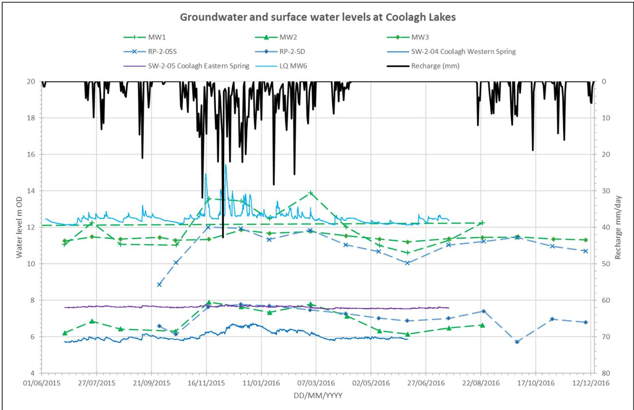
**Plate 10.5 Groundwater and Surface Water levels at Coolagh Lakes**
