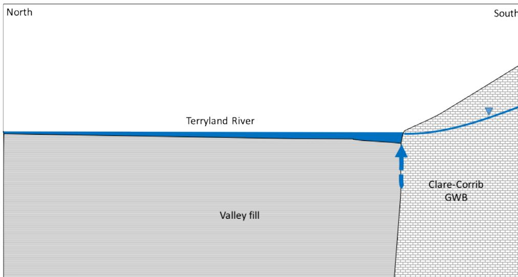
**Plate 10.14 Schematic north south Cross-section through Terryland River showing the Operation of the Estavelles at Pollavurleen West and East during High Groundwater Levels**
