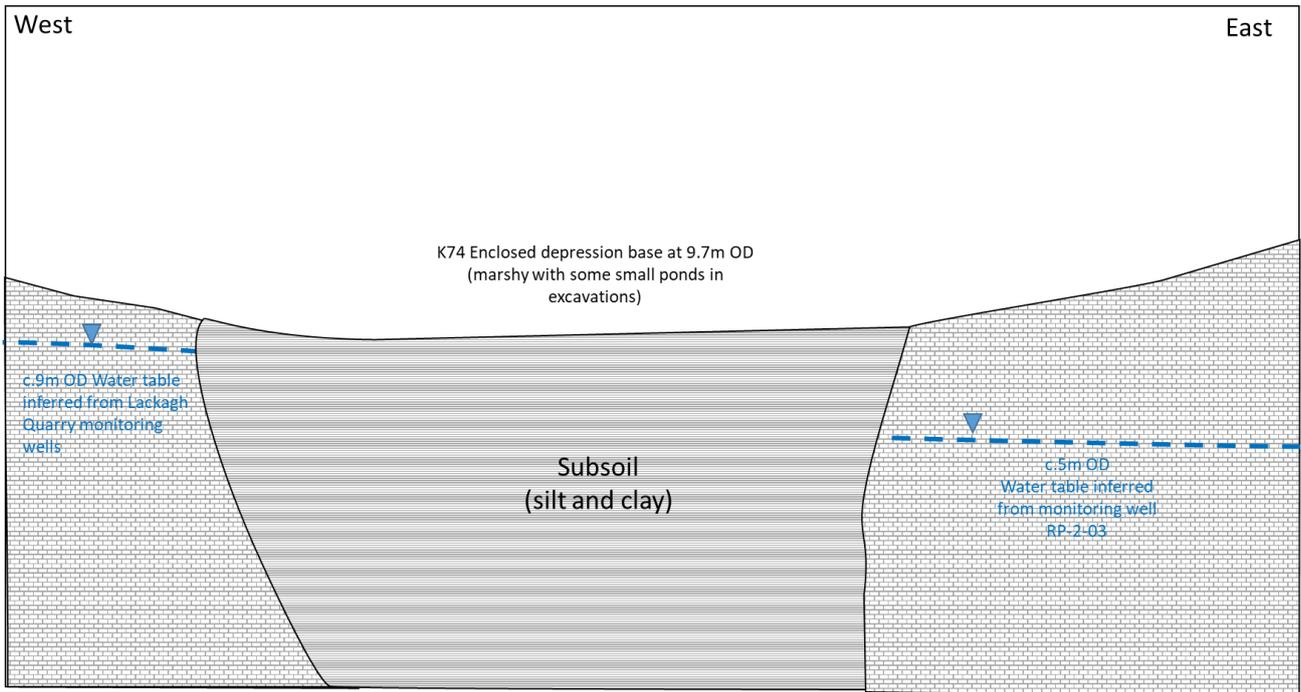
**Plate 10.13 Schematic east west Cross-section through Feature showing the Interaction of Groundwater with the Feature during Low Groundwater Levels**
