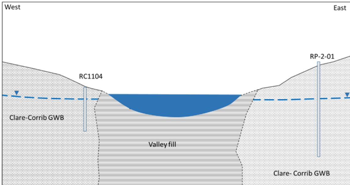
**Plate 10.8 Schematic east west Cross-section through Ballindooley Lough showing the Interaction of Groundwater with the Lake during Low Groundwater Levels**
