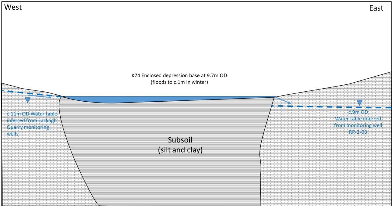
**Plate 10.12 Schematic east west Cross-section through Feature showing the Interaction of Groundwater with the Feature during High Groundwater Levels**
