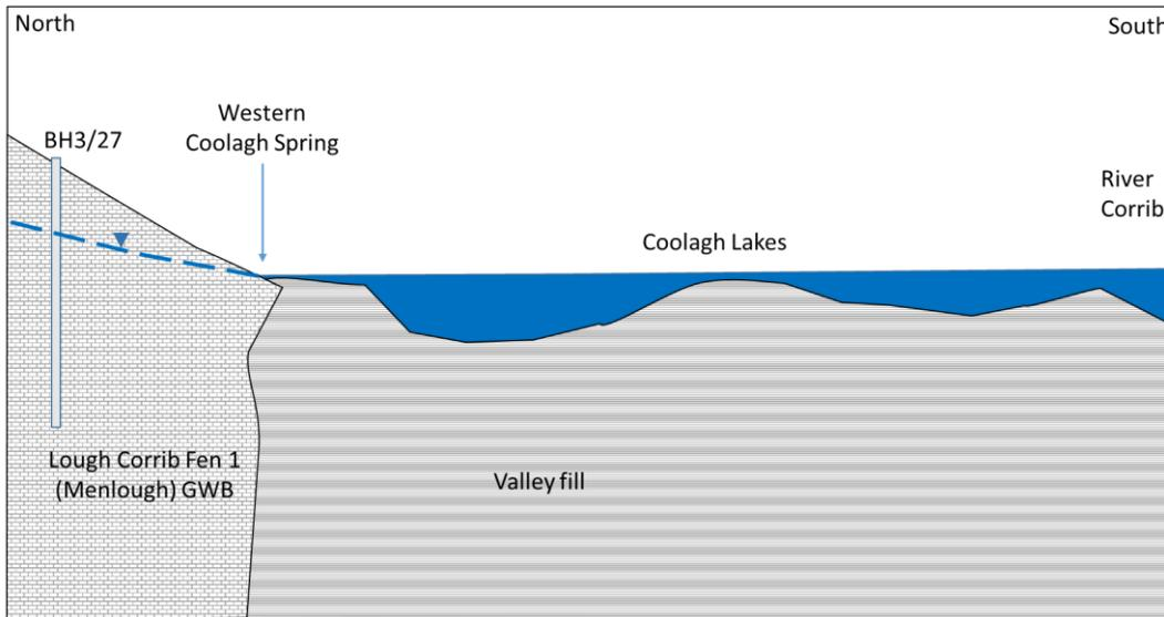
**Plate 10.3 Schematic north south Cross-section through Coolagh Lakes (Groundwater High)**
