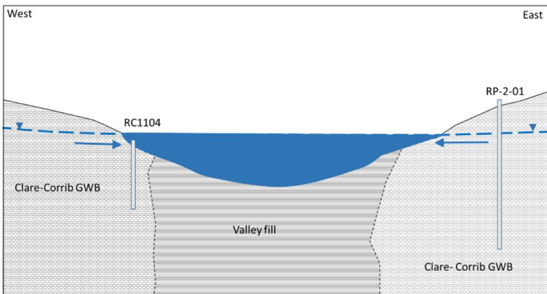
**Plate 10.7 Schematic east west Cross-section through Ballindooley Lough showing the Interaction of Groundwater with the Lake during High Groundwater Levels**
