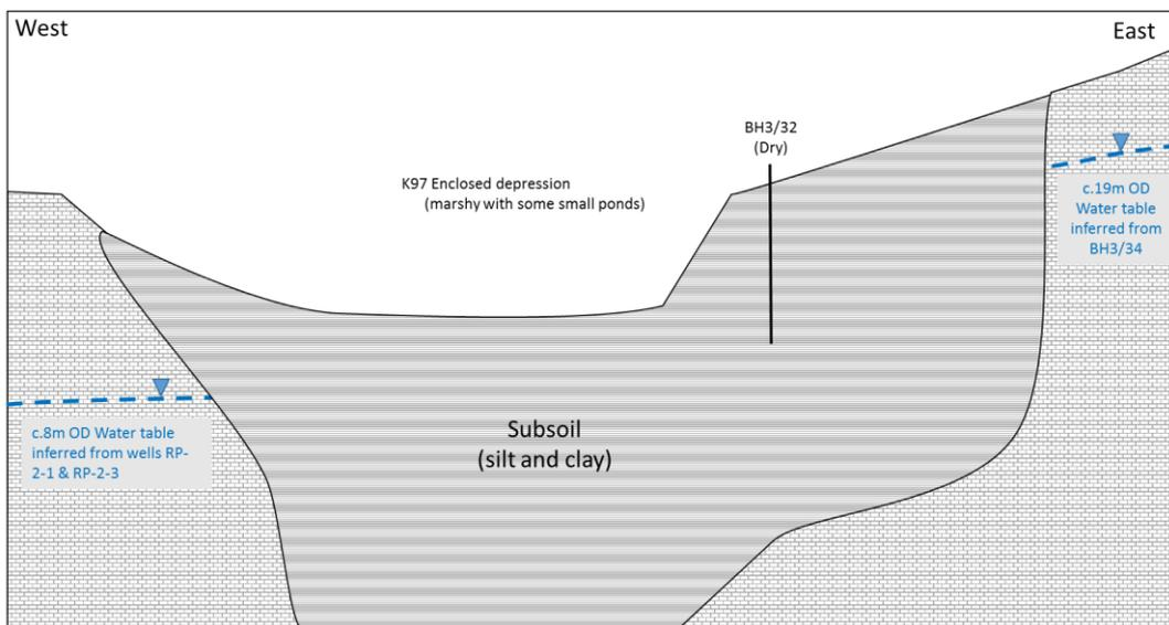
**Plate 10.11 Schematic east west Cross-section through Enclosed Depression K97 showing the Interaction of Groundwater with the Feature during Low Groundwater Levels**
