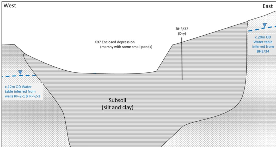
**Plate 10.10 Schematic east west Cross-section through Enclosed Depression K97 showing the Interaction of Groundwater with the Feature during High Groundwater Levels**
